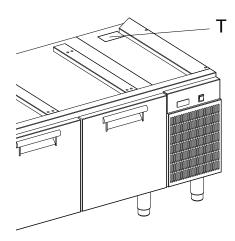
To connect the grill drain to the discharge pipe remove the precut panel "T".
